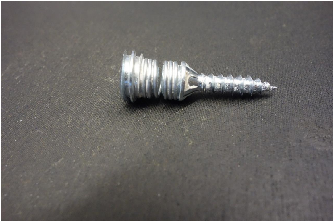
Picture 4 – The special screw in the measurement in enclosure 2.
