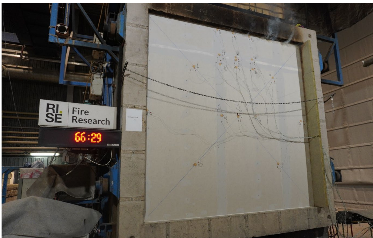
Test specimen after 66 minutes of the test.
