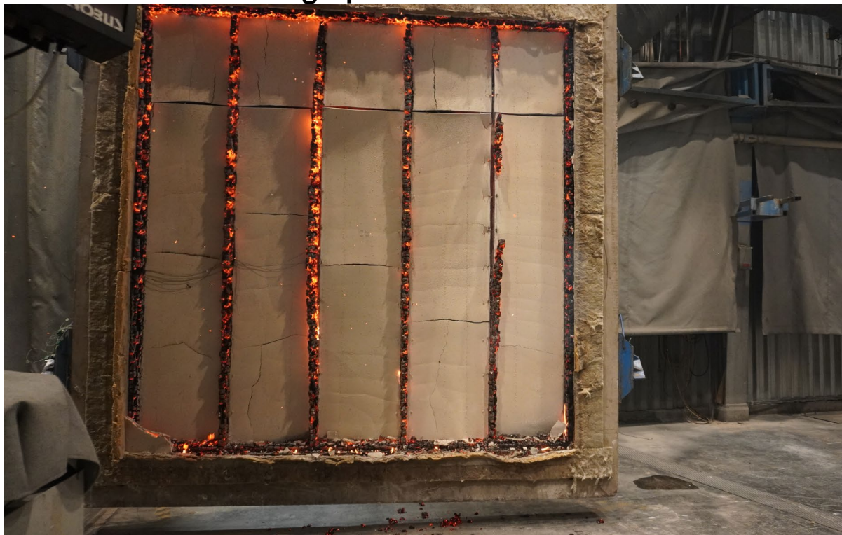
The fire exposed side of the specimen after the test.
