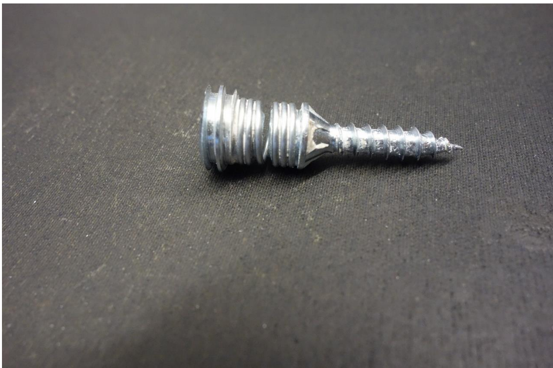
Picture 1 – The special screw used in the test with the furring in enclosure 1 and 3.
